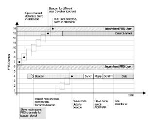
Fig. 2. Example of spectrum access behavior of the CIREN system
