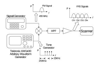
Fig. 4. Occupied channels test setup
