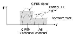
Fig. 6. Signal location for vacancy time measurement
