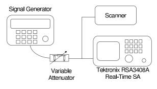
Fig. 3. Sensitivity test setup
